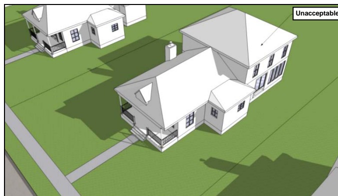
Unacceptable: A large mass occupies most of the rear yard and overwhelms the original structure.
